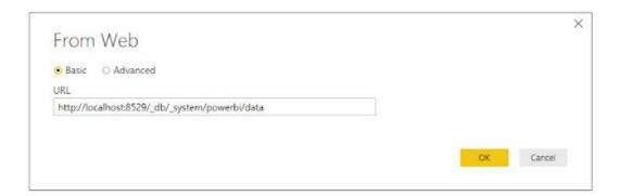
For example, if we have a local copy of ArangoDB running on our machine, the Power BI connector was installed at /powerbi and the name of the collection we want to import is data, our URL looks like this: http://localhost:8529/\_db/\_system/powerbi/data
